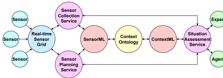
Figure 2: From sensor data to context in situation representation.
